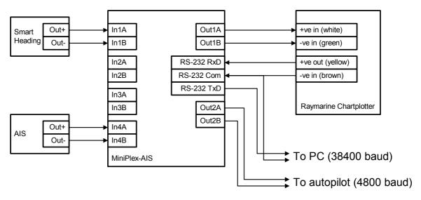
The picture above shows a typical configuration where the data of a heading sensor operating at a standard NMEA communication speed of 4800 baud is combined with the data of an AIS receiver/transponder operating at a communication speed of 38400 baud. The combined data is sent from NMEA Out 1 to the NMEA input of a Raymarine® chartplotter, which the NMEA port set to AIS.
