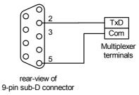
The serial port is galvanically isolated from the multiplexer to prevent ground loops and excessive currents that could otherwise destroy the multiplexer or the serial port of the connected computer.
