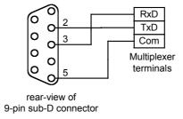
The RS-232 interface is set to 4800 baud when shipped. It can however be set to any speed in the range from 4800 to 38400 baud using the MPX-Config utility.
