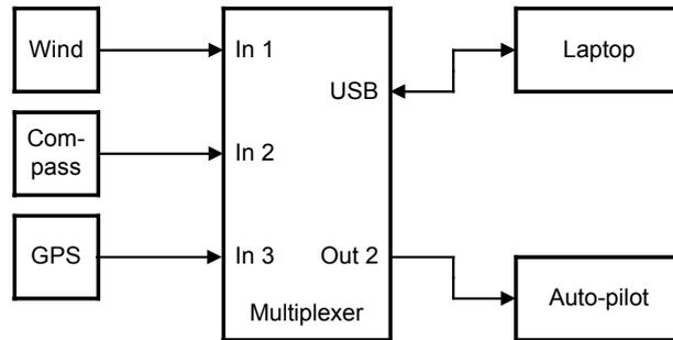
When the laptop is connected, it will receive all information from the instruments and the running navigation software is able to calculate the course to steer and drive the autopilot accordingly. Because the laptop is sending NMEA data, the multiplexer is in server mode and the autopilot will therefore receive information from the laptop only.
