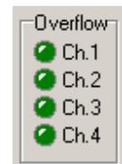
The overflow indicators on the MPX-Config screen can also be used to determine which channel is causing the overflow. The LED corresponding to the compass channel will be lit almost continuously. See the section **Operation** for ways to prevent an overflow.
