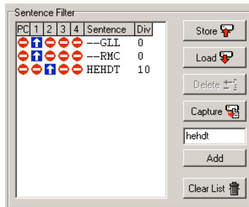
second, and the multiplexer or a connected device is suffering from an overflow, you can enter a 5 in the divisor column. The effect is that every fifth sentence will be passed while all others are blocked. This brings the sentence frequency down from 10 to 2 sentences per second.
